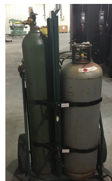
Figure 3-9: Portable Gas Tank Set
