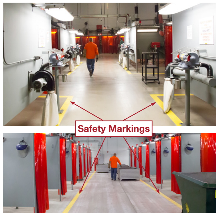
Figure 2-19: Bright Yellow Safety Markings on the Floor Designate Work Areas
