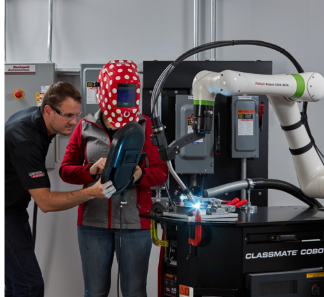
Figure 2-24: ClassMate® Cobot Robotic Welding Cell
