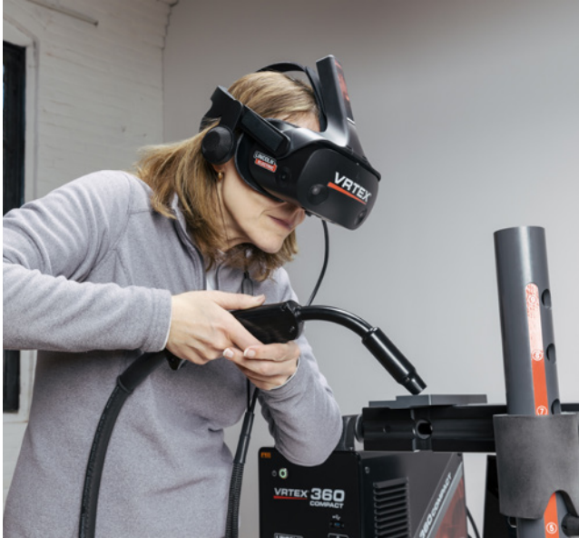
Figure 2-23: VRTEX® 360 Compact Portable Virtual Reality Welding Simulator Featuring GMAW
