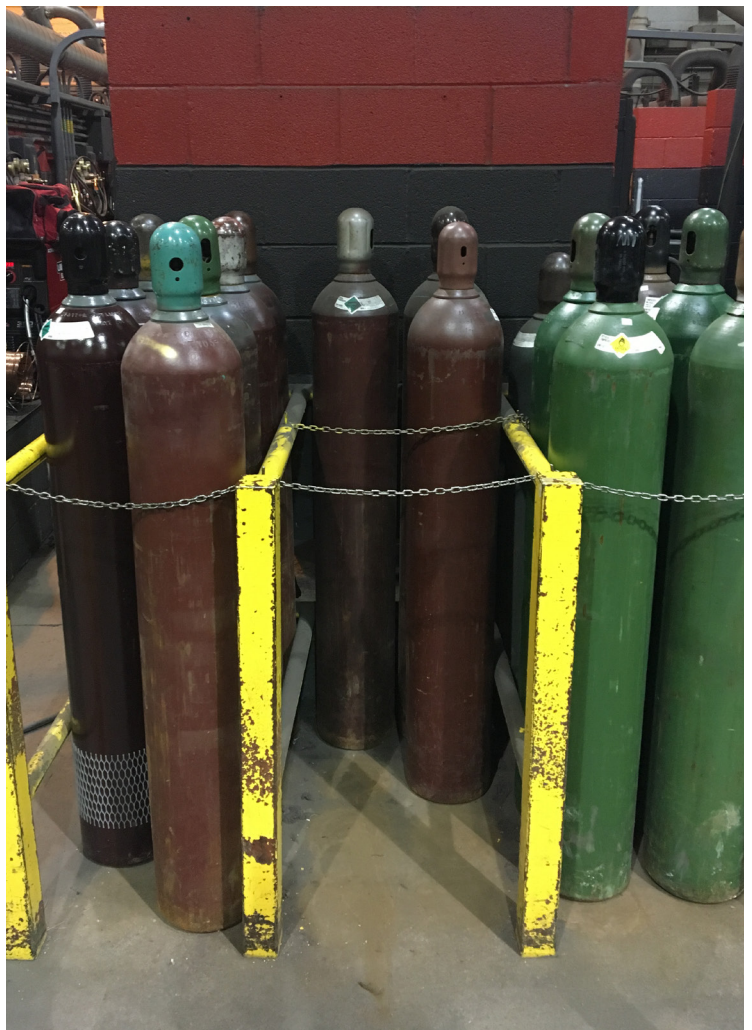
Figure 2-15: Inert Gas Cylinder Storage
