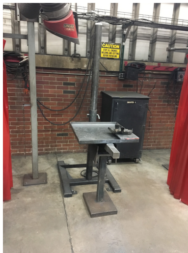
Figure 3-7: Booth Setup with Pole, Clamp, Exhaust
