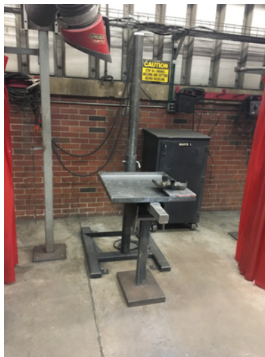
Figure 3-7: Booth Setup with Pole, Clamp, Exhaust
