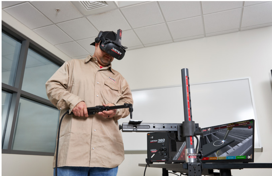
Figure 2-29: VRTEX® 360 Compact Virtual Reality Welding Trainer featuring optional Oxyfuel Cutting
