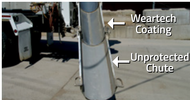
After 13 months in service, the Wearthech chute has 75% of coating thickness present and the aluminum base is 100% intact.
