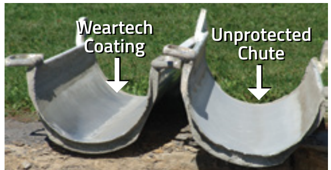
The unprotected chute shows severe wear from abrasion and erosion, leaks at the seams and must be removed from service.
