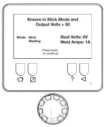
New PCB Calibration - Left Side Display (Single Mode)
