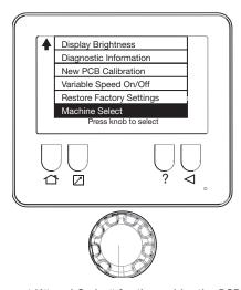
Enter the correct K# and Code # for the welder the PCB is being installed on. K# and Code # can be found above the top name plate("Machine Information Above"). Failure to enter the correct K# and Code # may result in permanent damage to the welder.
