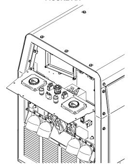
Locate VRD switches (as marked in Fig A.2) on both PC control boards. Left position on each switch indicates "OFF" state; right position on each switch indicates "ON" state. PC Control Board on the left is for settings for the left user. PC Control board on the right is for settings for the right user.
