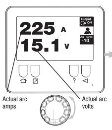
Stick Welding Basic 5 seconds after arc goes out
