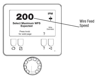
Note: Select the maximum wire feed speed (WFS) that will be used during the welding session to ensure power output to the wire feeder is sufficient.
