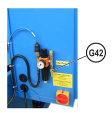
Connect the compressed air pipe to the filter located on the side of the electric unit on **G42**
