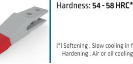
(\*) Softening : Slow cooling in furnace at 850°C Mixers Hardening : Air or oil cooling at 950 - 1000°C
