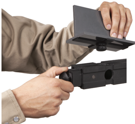
Figure 15 – Coupon insertion / removal
