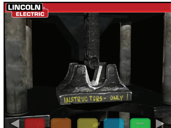
Figure 84 – Completed bend test
