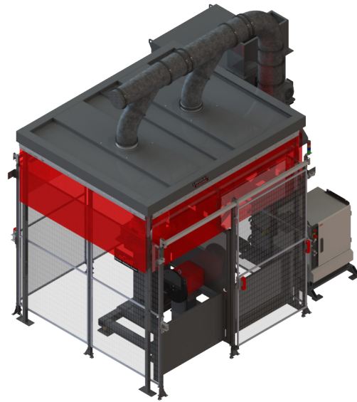
AD2532-4 eCELL HS water-cooled system with optional fume extraction hood
