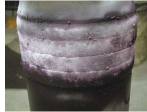
Dye penetrant testing proves Guardian HB's superior cracking resistance
