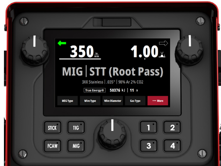
PIPEFAB™ system navigation home screen
