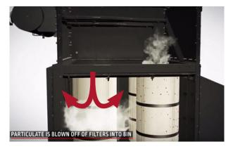
The pulses remove particulate from the filters, which falls into the dustbins below.
