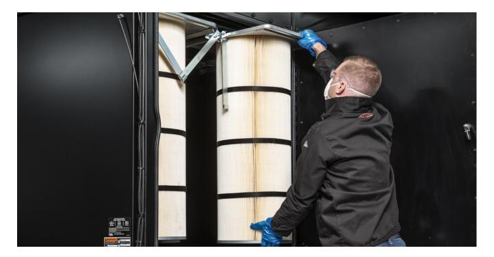
Prism Filter Banks are equipped with automatic filter cleaning, but over time filters will become saturated with particulate and will need to be replaced. These systems are designed for quick and easy filter maintenance:
