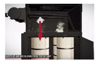
Systematic pulses of air are released from the air compressor above the filters.
