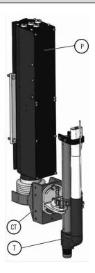
The torch impact safety system  $\mathbf{CT}$  is a machine protection device that is mounted between the tool holder  $\mathbf{P}$  and a cutting torch  $\mathbf{T}$ .
