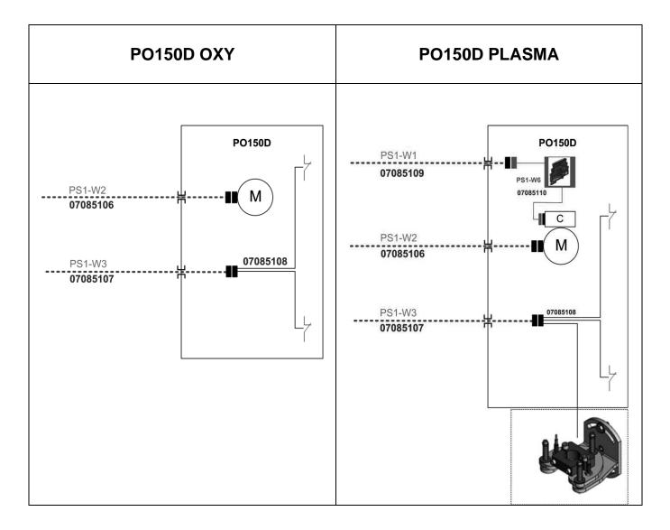
The connectors have foolproofing to avoid reversed connections.
