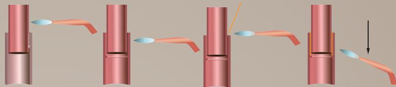
Fig. 12 Tube-heating sequence
