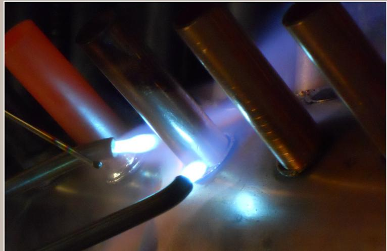
*Brazing is primarily defined by the ability of the molten filler metal to spread and adhere to the base metal (wetting), and its ability to flow into the tight spaces between parts (capillary action).*
