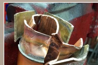
**Fig. 4** Peel test results
