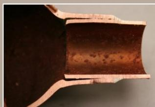
**Fig. 2** Sectioned brazed joint showing lack of filler metal penetration
