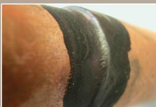
**Fig. 1** Exterior view of a copper-brazed tube
