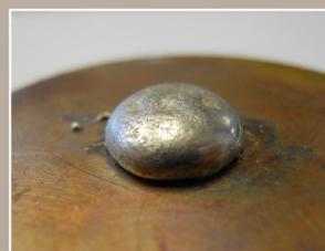
**Fig. 5** Solder nonwetting without flux
