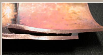
**Fig. 10** Insufficient penetration
