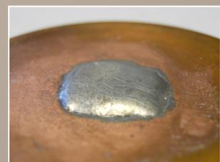
**Fig. 6** Solder wetting when flux is applied
