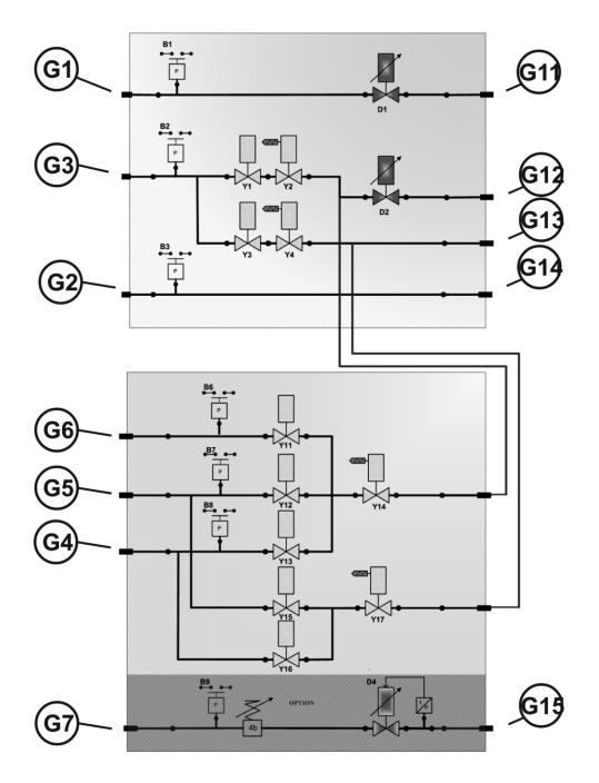
The part between G7 and G15 is added when this option is installed.
