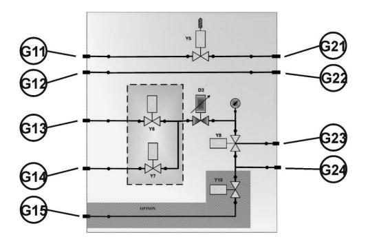
The G15 line is added when this option is installed.
