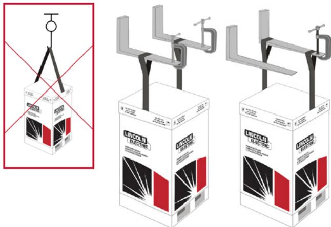
8. Lift the box straight up off the wooden master pallet.
