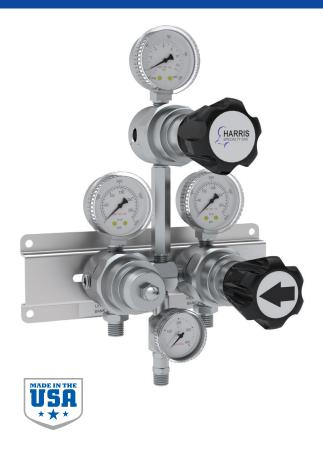
The SG 900 BR / SG 905 SS semi-automatic high purity switchover prevents downtime by automatically switching gas supply from the primary cylinder bank to the reserve cylinder bank. The user resets the primary bank by turning the knob. Manual adjustment of the individual regulators is not required. All systems include a line control regulator.
