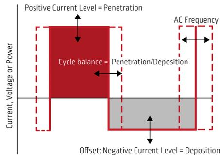
With AC wave form, increase deposition rate up to 50%.
