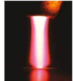
The contribution of energy necessary for welding is ensured by an electric arc in an atmosphere of plasmagene neutral gas. This arc established between an infusible electrode and the parts to be assembled is forced through a nozzle which constricts it mechanically and pneumatically. This welding process is used for welding of carbon steel, stainless steel, duplex, titanium, Inconel, nickel and alloys...
