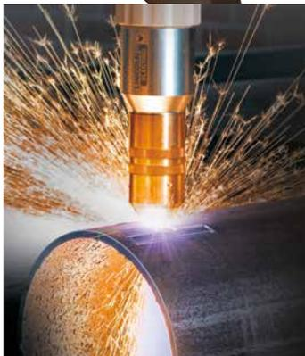
**Plasma cutting system with tube cutting**
