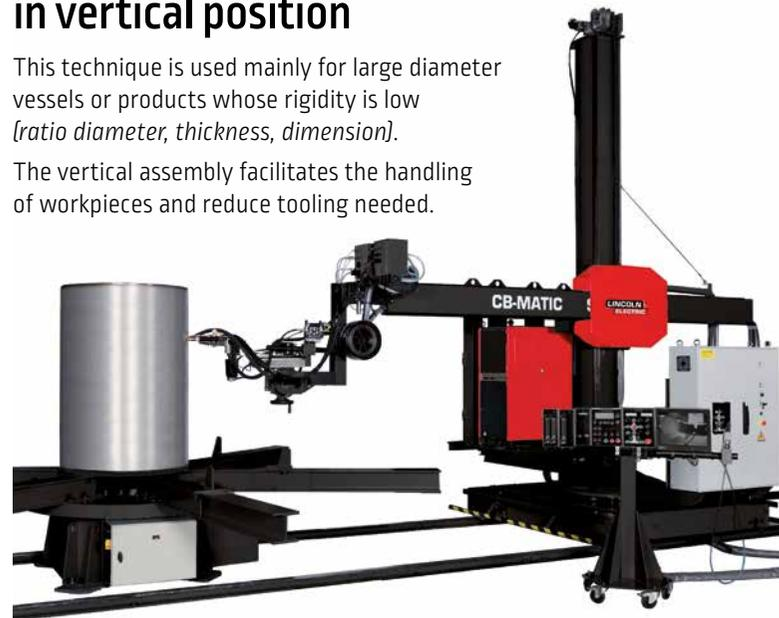
**Column and boom with turntable** for longitudinal and circumferential welding:
