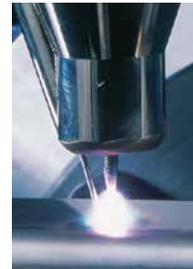
Based on principle of TIG process, an additional filler metal is fed through the nozzle directly into the arc with an angle of 20° to the electrode. This concept guarantees a high deposition rate and an efficient metal transfer. This welding process is used for welding of carbon steel, stainless steel, titanium, inconel, electro-galvanized coated steel (*brazing*)...
