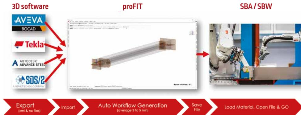
It only takes a few minutes to auto-generate the workflow without programming or teaching the robots, and it doesn't stop there. The significant time and cost savings are during the assembly process, demonstrating a system that can be up to 10 times faster than a traditional manual fitting process.
