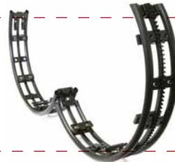
**Flat Track 48"** [1219 mm] can be bolted together to create length tracks as required.
