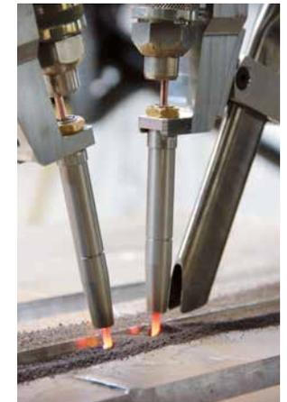
LSO combined to AC wave form, increase deposition rate up to 100%.
