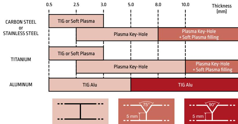
Maximum thickness which can be welded in a single pass is reduced for:
