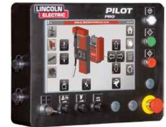
**PILOT PRO Plus** controller for a centralized management of the machine.
