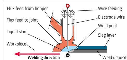
Similar to MIG/MAG welding, SAW involves the formation of an arc between a continuously fed wire electrode. Covering flux is used to generate protective gas and slag protecting the weld metal. The flux can also help donate alloying elements. It is dedicated mainly for flat and fillet welding. This process is generally used for the welding of materials as carbon steel and stainless steel.
