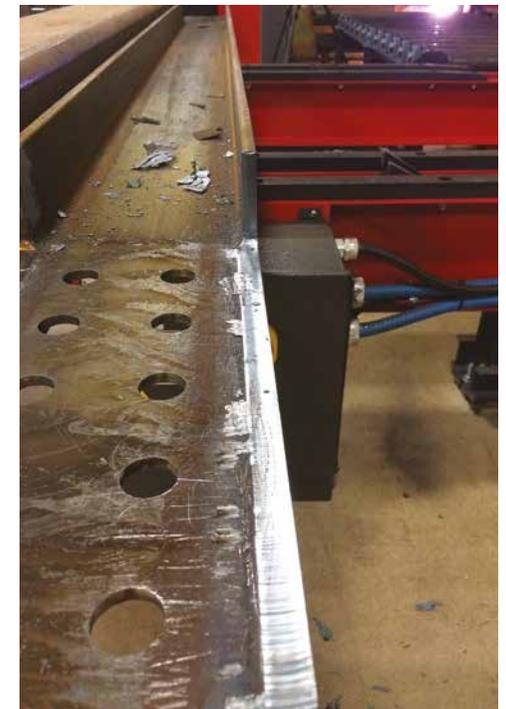
This CE certified system takes in your drawing files and automatically processes beams, channels, angles, square and rectangular tubes, as well as plate, all on one machine. In addition, the machine produces bolt holes that are EN1090 compliant.
