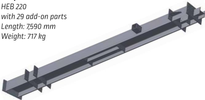
\* Dimensions of main beams and add-on parts may vary according to the machine type.
