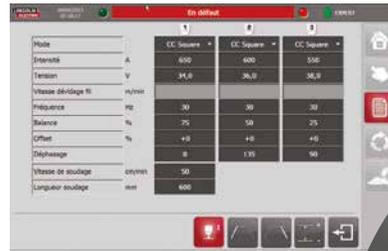
Clear display of welding parameters
