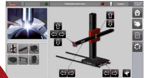
Graphic display of the machine and welding head
