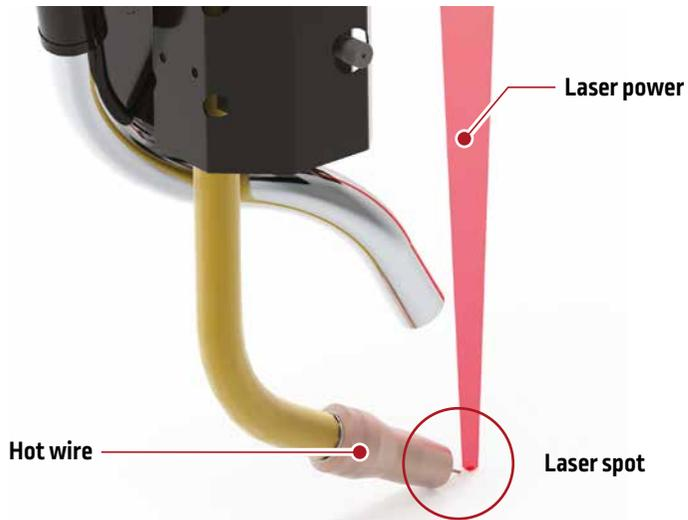
This process is an arc-free, hotwire laser process designed to increase deposition rates and travel speeds by heating the wire to a certain degree before entering it into the laser beam.
