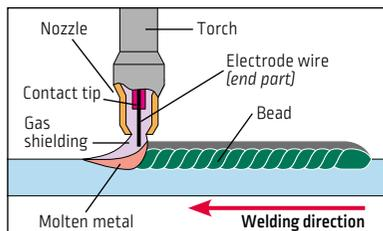
An electric arc forms between a consumable wire electrode and the workpiece (*metal*) which heats the workpiece metal causing them to fuse. The arc and weld pool are shielded by an inert or active gas. Metal is transferred in the form of drops through the arc towards the workpiece. This welding process is used for welding of carbon steel, stainless steel, aluminium, copper...
