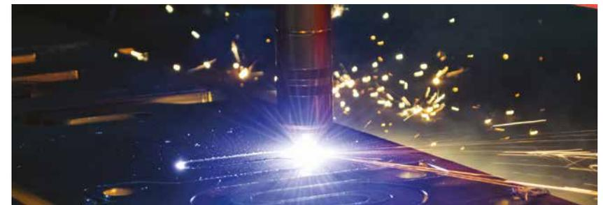
\*Cutting at 140A on PythonX STRUCTUAL using the FineLine® 300HD System
