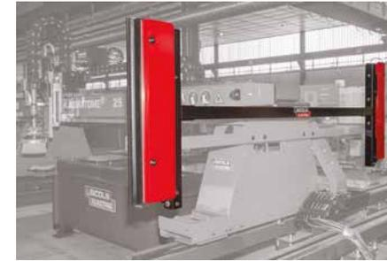
Operator protection customizable depending on the implementation of the machine inside the customer workshop to ensure safety and be compliant with machine regulation.
