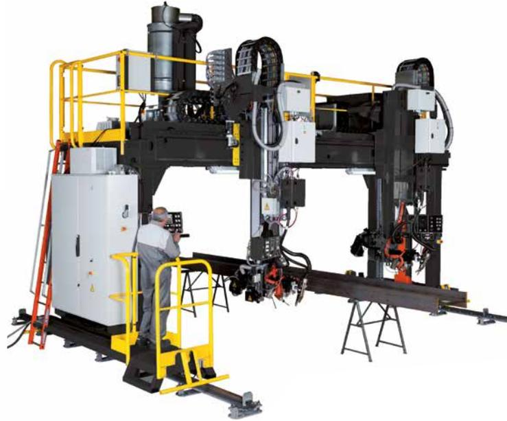
**MIG MAG welding aluminium Gantry** with two torches to answer applications requiring a high level of productivity with large pieces such as the manufacture of railway wagons.
