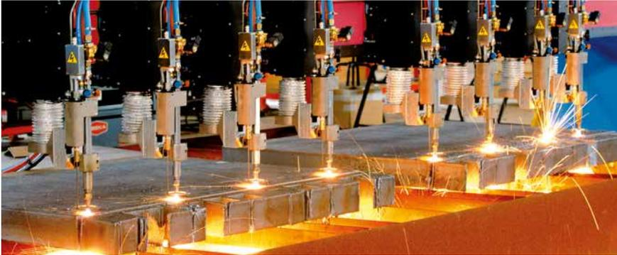
A well adapted software help increases the automation and the return on investment of machines fitted with the CNC. Lincoln Electric can supply software specially designed for thermal cutting CAD, pressure vessel shapes developed flat, interleaving, plate stock control, communication, translation of external files and files produced by other CAD systems [DXF, DWG, DSTV...].
