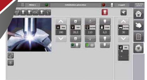
Quick access and display of welding functions
