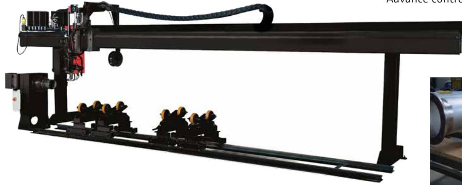
**Mechanisation machine** with plasma process and Pilot Advance control to weld pipes with elbows and flanges.
