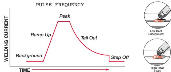
**Pulsed MIG Mode** varies weld current between peak (high heat) and background (low heat) current to provide better control of heat input, which minimizes warping and burnthrough on thin materials. Pulsed MIG also enables flat, horizontal, vertical up, or overhead welding without a slag system. Optimized GMAW-P waveforms are readily available to use on aluminum, carbon steel, high strength low alloy steel, stainless steel, and nickel alloys.
