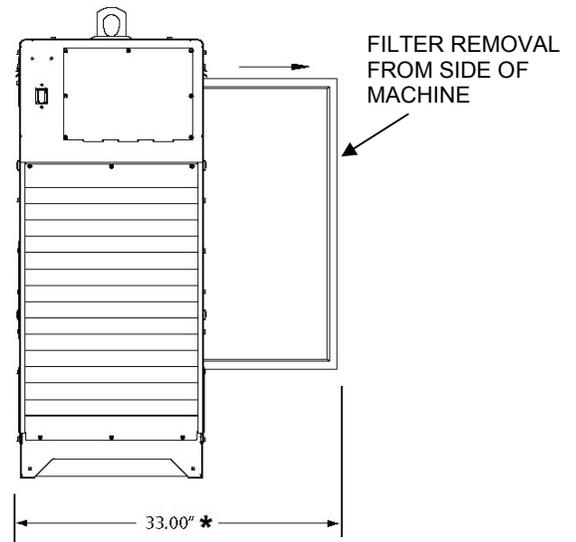
\*: 33.00" width needed for filter maintenance access.
