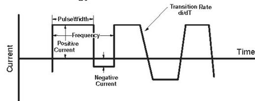
Depending on the process, different parts of the output waveform and wire feed speed may be modulated at varying rates to achieve a smooth and stable arc.
