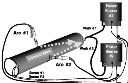
**NOTE: DeviceNet cables should not be routed with weld cables, wire drive control cables, or any other current carrying device that can create a fluctuating magnetic field.**
