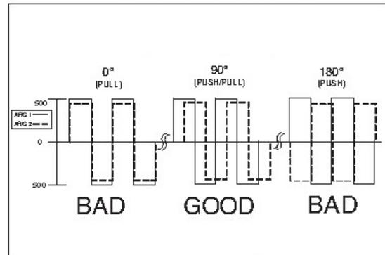
Best results obtained by alternating and equalizing the duration of magnetic forces between adjacent arcs.
