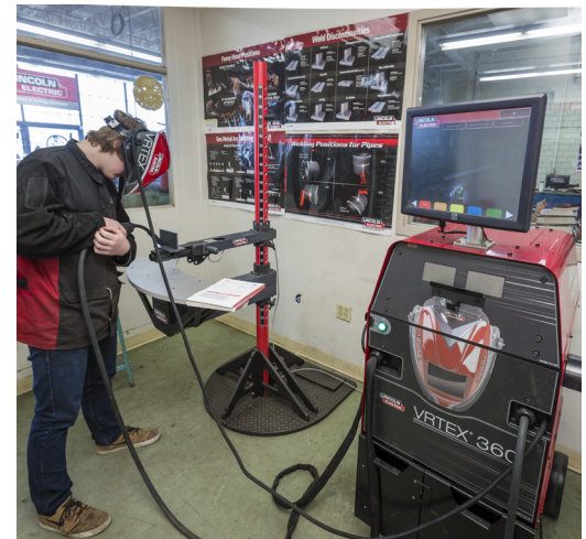
Parma Senior High uses the Lincoln Electric VRTEX® 360 virtual reality welding simulator system to allow students to practice technique without wasting material, electrodes or shielding gas.
