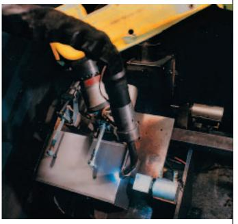
combines a FANUC Arc Mate 100i, 6-axis robot with Lincoln's Surface Tension Transfer (STT) power source. The System 40 is a "drop-in-place-and-plug-in" work station with a small, forklift-compatible footprint. For DeWys, that translated to easy installation, plus the ability to move the robot around the shop when necessary.
