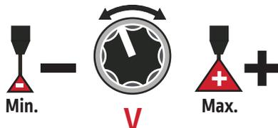
4. Synergic Weld modes improve the ease of set-up by pre-selecting an ideal voltage based on the selected WFS. The user can then fine tune their Voltage setting based on their personal preference and can easily see whether they are above or below the nominal setting.
