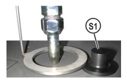
Set the probe ring with the spacer **S1** and mechanically adjust the probe to leave 5mm between the probe and the sheet, over the entire probe
