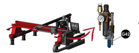
Connect the compressed air pipe to the filter located on the side of the electric unit on **G42**.
