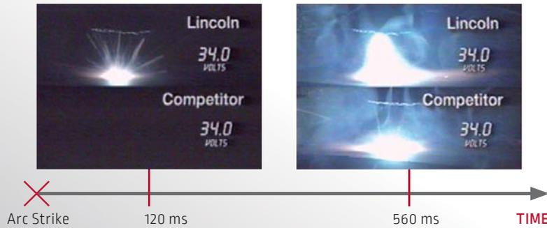
Arc establishment comparison of new engineered premium wire against competition - clearly demonstrating faster arc establishment
