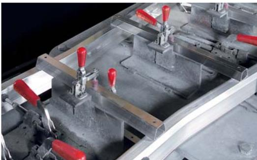
The level of efficiency of automation depends on the thoughtful design of the fixturing for maximum productivity. Many productivity gains are realized at the design stage and while parts fixturing performs a role that is simple, good fixture design is critical to the success of a robotic welding system.
