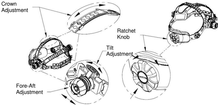
**HEAD SIZE ADJUSTMENT:** HEADGEAR TIGHTNESS is adjusted by pushing in the Ratchet Knob and turning to adjust for the desired head size. This knob is located at the back of the helmet. **HEADGEAR CROWN ADJUSTMENTS** are made by adjusting for comfort and snapping the pins into the hole to lock securely in place.
