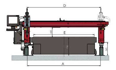
Dimensions on a standard railway (Length 4500 mm). Additional roller railway with 3 m or 1.5 m elements.
