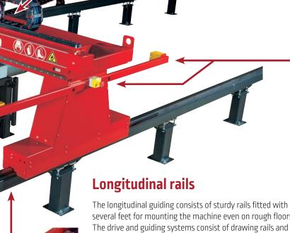
several feet for mounting the machine even on rough floors. The drive and guiding systems consist of drawing rails and racks facing outwards.
