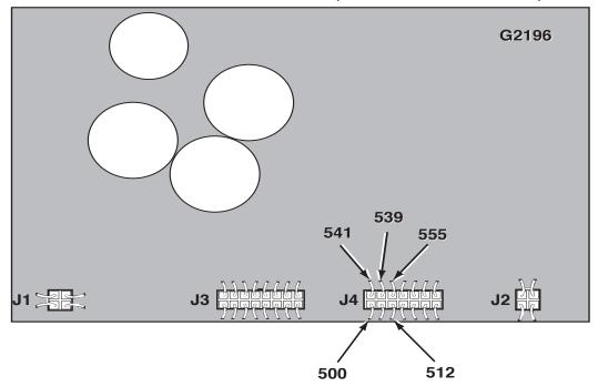
FIGURE F.10 - CONTROL PC BOARD (CODES 9812 AND BELOW).
