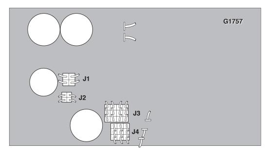
For codes 9812 and below, remove the contactor coil leads and plug J7 from the contactor PC board. See Figure F.17. Also for codes 9812 and below, remove plug J3 from the control PC board. See Figure F.18.
