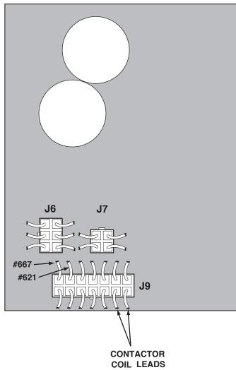
4. Apply 12 VDC to the contactor coil leads.
