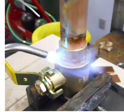
2 Heat valve – move torch to heat all sides of valve. Begin heating away from the fluxed area to preheat the part. Then direct the flame to the to where you'll apply solder.
