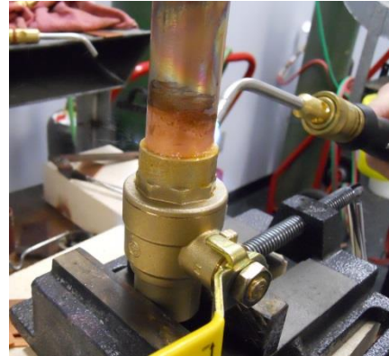
2 Heat valve – move torch to heat all sides of valve. Begin heating away from the fluxed area to preheat the part. Then direct the flame to the to where you'll apply solder.
