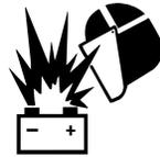
**GASES FROM BATTERY** can explode.
