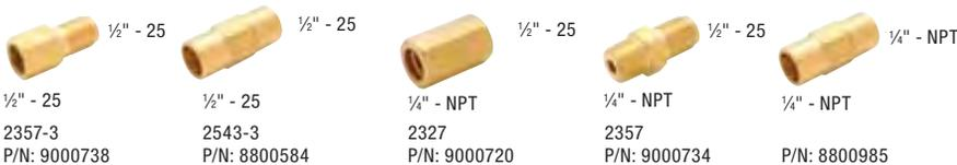
Multiple arrangements of 2290-H Heating Tips can be assembled using Harris coupling 2327, nipple 2357 and standard 1/4" pipe fittings when wider bands of heat are necessary. Capacity of K-43 heating torch is 5 NO.1-H tips. Use coupling 2543-3 to couple 2393 Tip Tubes for extended reach. For extended tube and tip life, use adaptor 2357-3.
