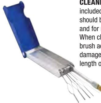
**CLEANING INSTRUCTIONS:** The wire brush included with tip cleaner E-9 (P/N: 9000160) should be used for cleaning preheat slots and for removing spatter from the tip face. When cleaning the preheat slots, do not brush across the slots as this motion can damage the slots. Always brush along the length of the slot to remove dirt or spatter.
