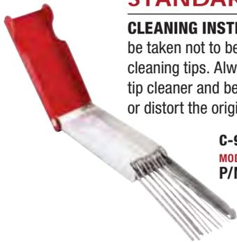
**CLEANING INSTRUCTIONS:** Care should be taken not to be too aggressive when cleaning tips. Always use the proper size tip cleaner and be careful not to enlarge or distort the original tip bore size.
