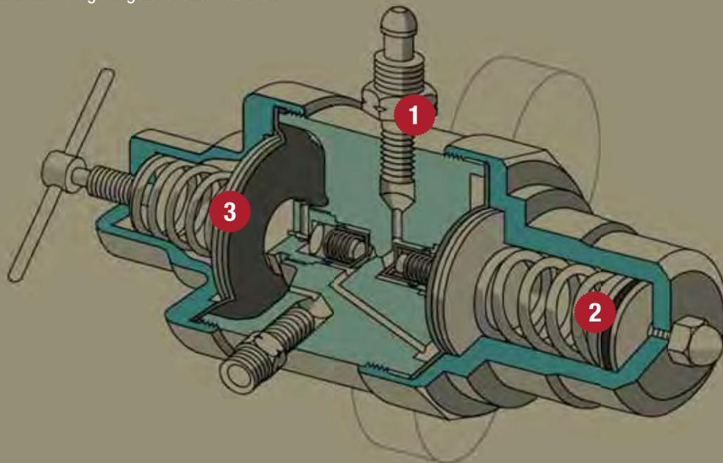
**1** INLET PRESSURE IS REDUCED IN TWO STAGES
