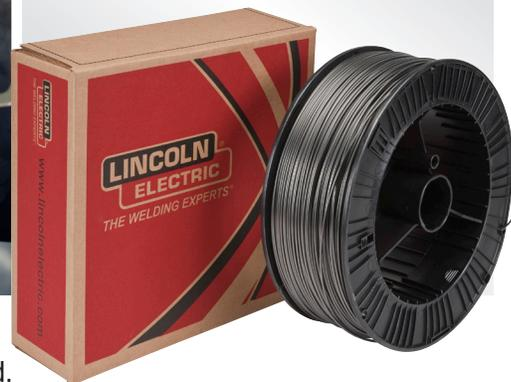
Metalshield® MC®-90 is a low alloy metal-cored wire designed for high strength welding where tensile requirements of 620 MPa (90ksi) are required. For an electrode designed to produce enhanced strength, high toughness, and H4 diffusible hydrogen weld deposits required in many applications, including pressure vessels – choose Metalshield® MC®-90.
