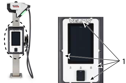
Figure 36 Replacing User Interface Seals
