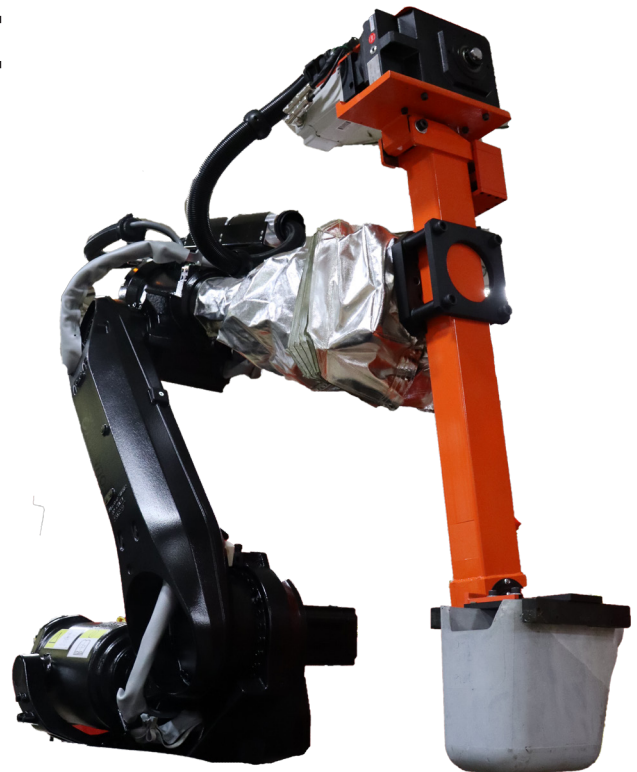
Rimrock 7 th Axis Ladle EOAT on ABB ® robot
