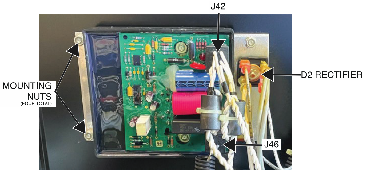
Figure F.2 – 40 VDC bus board plug and mounting hardware locations
