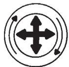
Rotate the filter while pulling straight out.
