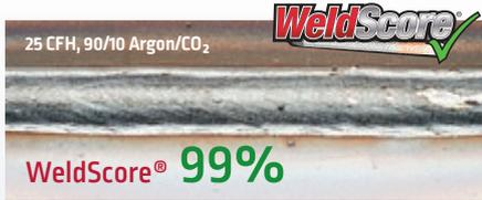
Acceptable Weld – Proper gas flow and coverage produces a good weld with no porosity.
