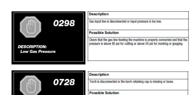
Check that the consumables are properly installed. Tighten retaining cap
