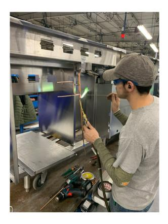
**PERFECT FLAME:** A worker uses the Perfect Flame<sup>TM</sup> to braze equipment on the production floor at Delfield. (Courtesy of Harris Products Group)
