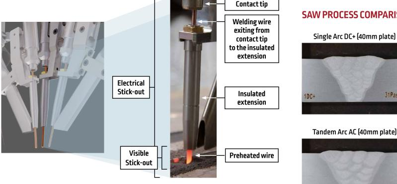
*Operator friendly: The visible stick-out remains the same as for the conventional process.* Only the electrical stick-out increases. It does not change his operating methodology.
