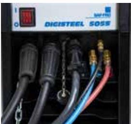
Cable connections on front (in standard) and back rear side (in option). Strain relievers on both ends to keep connections well protected.
