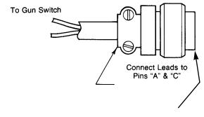
S12024-1 (L.E. Part No.) Amphenol AN3057-10 (or equiv.) S12020-6 (L.E. Part No.) Amphenol MS-3106A-18-11P (or equiv.)
