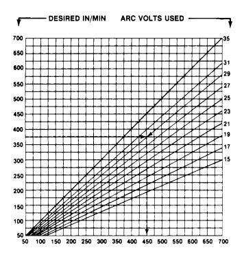
FIGURE B.3 CC WIRE SPEED SETTING
