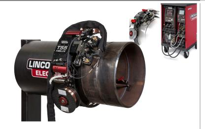
Orbital welding systems can be used to automatically weld pipe and tube in locations that are difficult to access or for critical applications.
