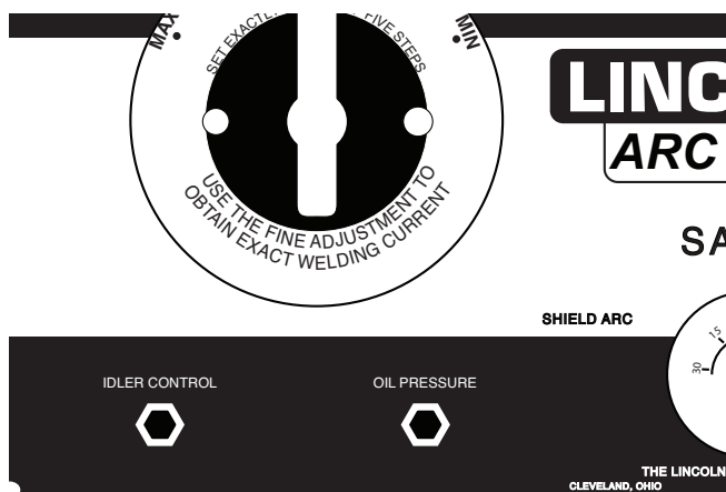
FIGURE 5 – Idler Control Switch.
