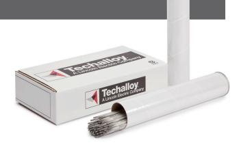
**Tech-Rod**® **347** electrodes are niobium stabilized stainless steel electrodes used for the welding of types 347 and 321 stainless and stainless clad steels. The addition of niobium reduces intergranular corrosion in severe operating conditions.
