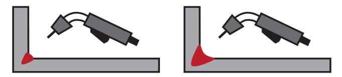
**Wire Feed Speed** - As your wire feed speed is increased the weld penetration increases, and as your wire feed speed is decreased, the weld penetration decreases. Notice the changes to the weld puddle in the image shown above.
