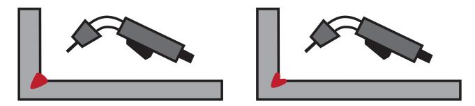
**Voltage** - Arc voltage affects the arc length. At the same wire feed speed, as voltage increases, the arc length gets longer and as voltage decreases, the arc length gets shorter. The length of the arc in turn determines the width and size of the arc cone. Notice the changes to the weld puddle in the image shown above.
