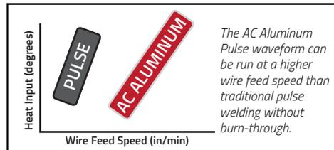
*The AC Aluminum Pulse waveform can be run at a higher wire feed speed than traditional pulse welding without burn-through.*
