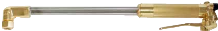
The genuine Harris H28 torch features a solid brass forged head that resists flashback damage, and triangular stainless steel tubes with brazed connections for added strength.
