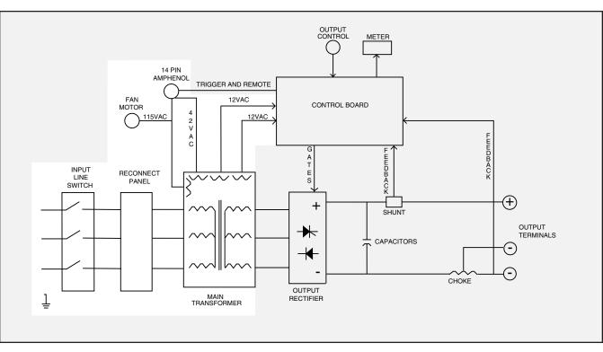
Figure E.2 - Input Line Voltage, Line Switch and Main Transformer
