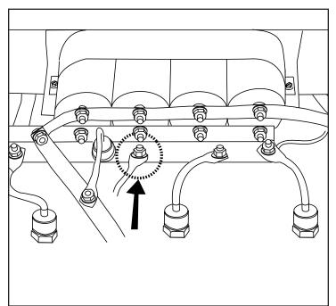
FIGURE F.13 - Procedure to disconnect the D5 diode pigtail from the negative capacitor buss.
