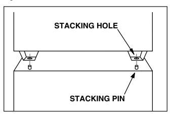
FIGURE A.1 - Stacking IDEALARC CV-300 machines.
