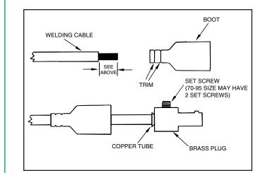
FIGURE A.6 - Installing Twist-Mate Cable Plug.
