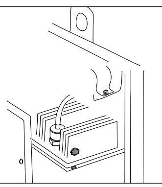
FIGURE F.15 - Heat sink test points.
