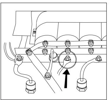
FIGURE F.6 - Procedure to disconnect the D5 diode pigtail from the negative capacitor buss.
