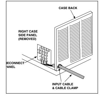
FIGURE A.2 - Input Power Cable Entry Connections and Reconnect Panel location.
