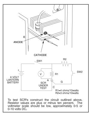
FIGURE F.16 - SCR Tester Circuit and SCR connections.
