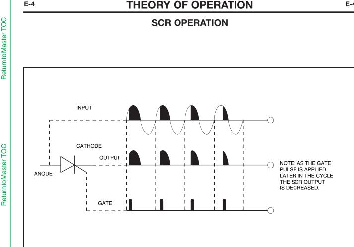
Figure E.4 - SCR Operation
