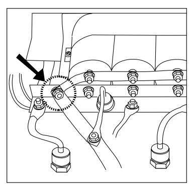
FIGURE F.5 - Procedure to disconnect the strap from the positive heat sink to the capacitor bank.
