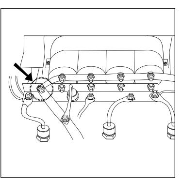
FIGURE F.12 - Procedure to disconnect the strap from the positive heat sink to the capacitor bank.
