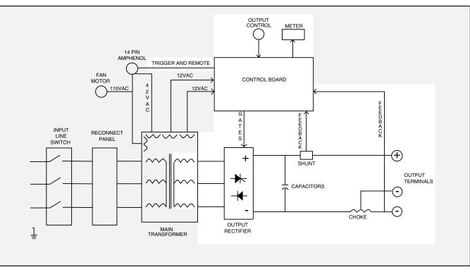
Figure E.3 - Output Rectification, Filtering, Control and Feedback
