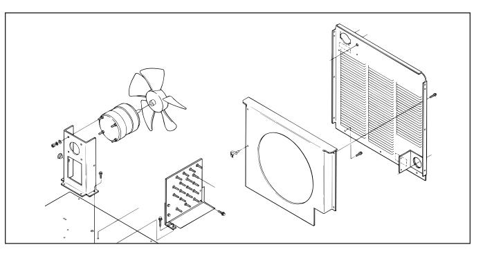
FIGURE F.25 - Fan Motor removal.
