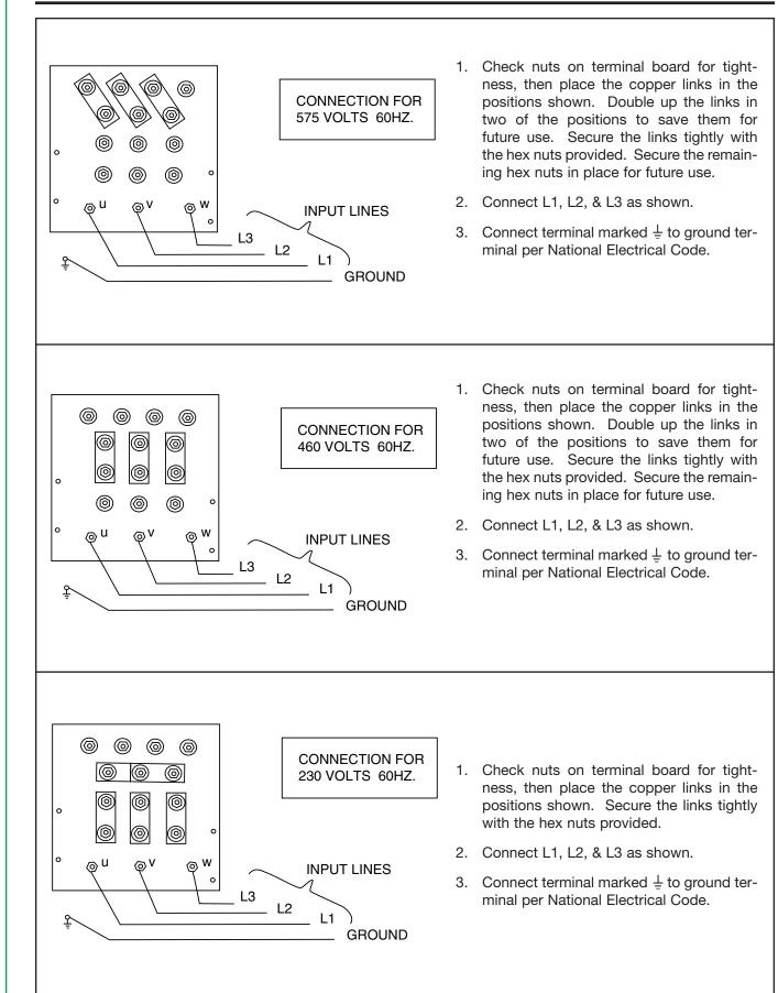
FIGURE A.5 - Reconnect Diagram for 230/460/575 voltage machines.
