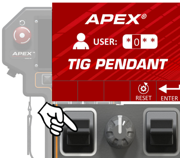
FIGURE 5A - Fast Movement Left Toggle
