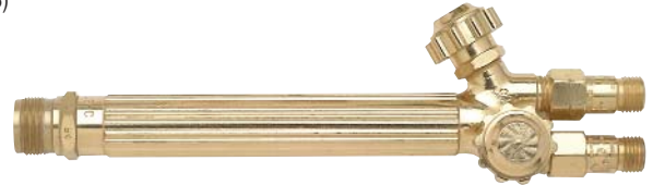
Model V-315C Length: 9 1/2"; Weight: 1.4 lbs. Cuts 6", welds to 1" (page 9)
