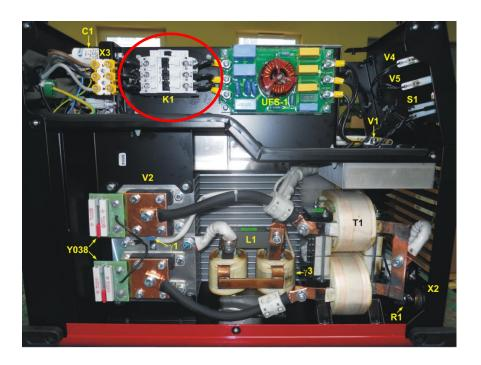
2. The new (big) contactor has to be installed on the horizontal machine frame, as shown into picture below (proper holes have to be done on the horizontal frame)
